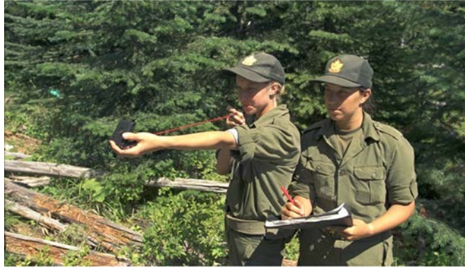
Figure 1 Determining a Magnetic Bearing
