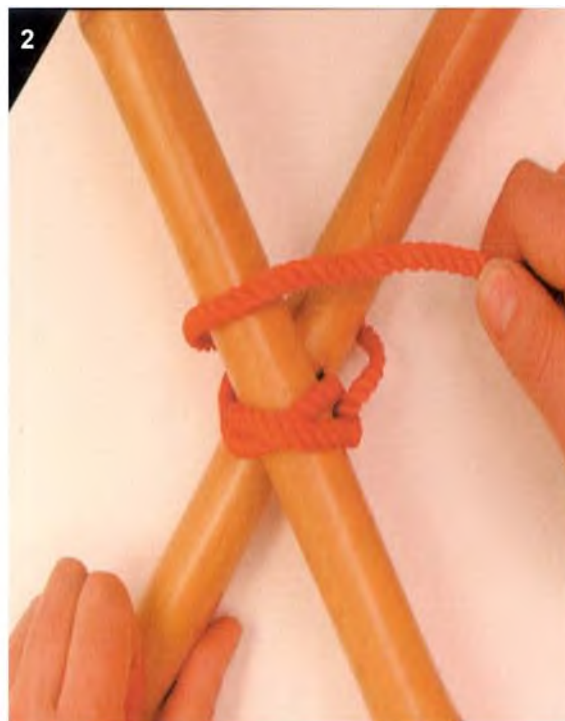
STEP TWO. MAKE A TURN AROUND THE TWO CROSSED POLES, PULLING THE TIMBER HITCH TIGHT.
